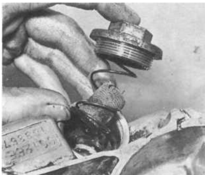
Strainer is easily removed for cleaning
