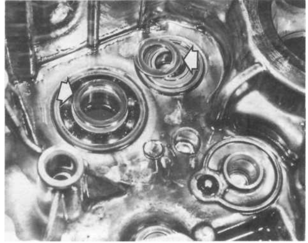
1 6.3b Do not lose these shims which may remain in case
