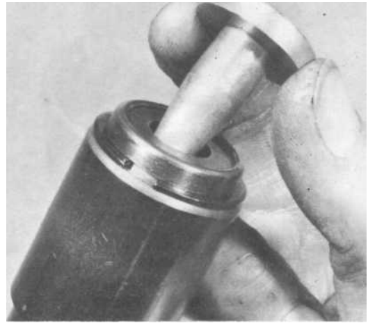
7.6c Do not omit restrictor, if removed
