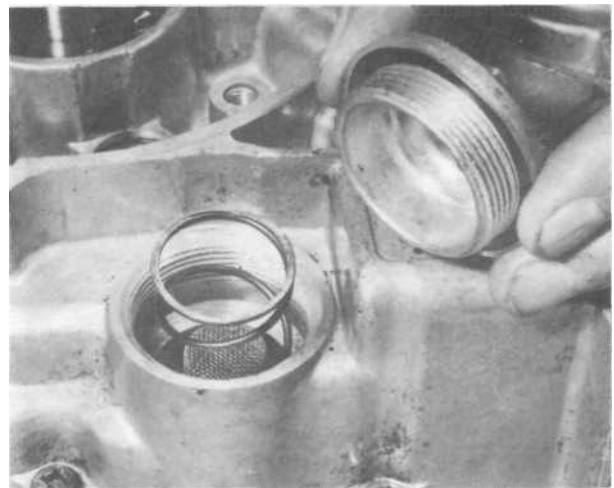
37.1a Refit gauze crankcase filter assembly
