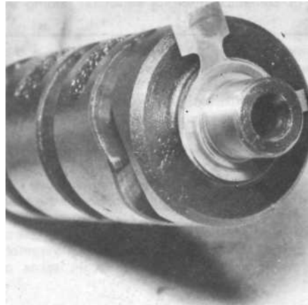
33.2a Do not omit the neutral switch contact during reassembly
