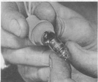
1.7g ... bulb is of bayonet type - always ensure correct wattage bulb is fitted
