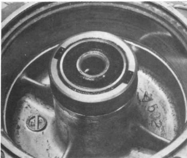
4.2 Examine the brake drum surface for signs of scoring
