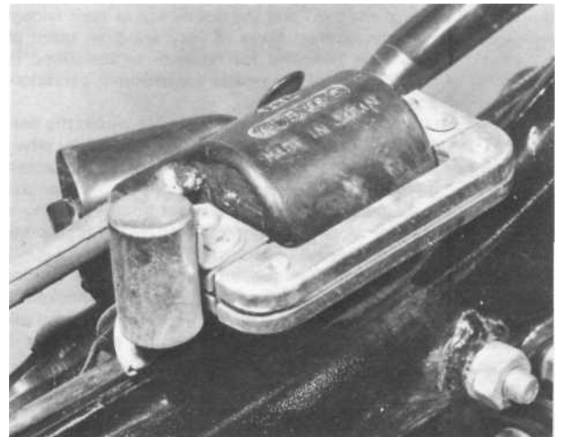
6.1 Coil and condenser are located beneath the fuel tank
