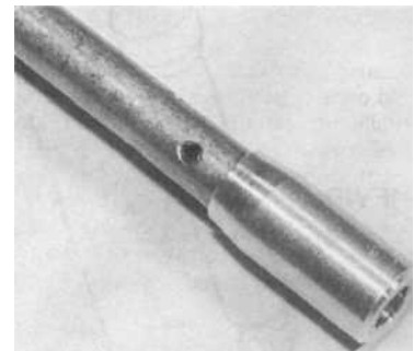
21.2c When damper rod projects from stanchion lower end, fit damper rod seat
