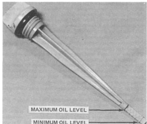
Dipstick shows allowable oil level range
