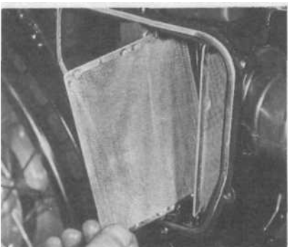
4.3 Note two flame traps - one is fitted next to filter element
