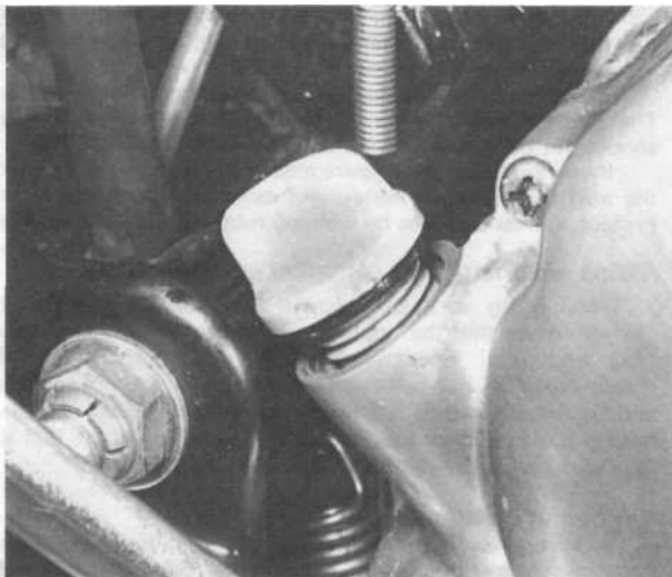
Rest dipstick in position to obtain correct reading
