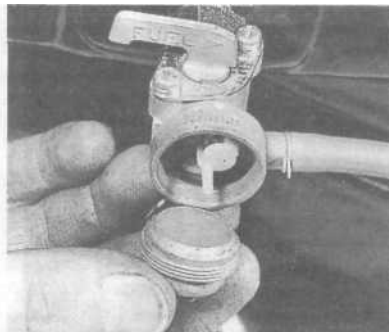
4.9b Do not overtighten filter bowl note sealing O-ring
