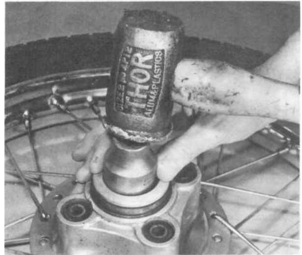
11.2c A large socket makes a useful drift
