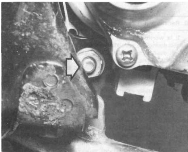
40.2c .. noting that lower nut is rather inaccessible
