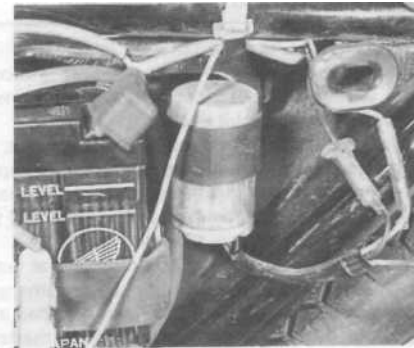
12.1 Flasher unit is rubber-mounted to rear of battery
