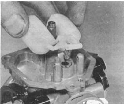
15.1 If float assembly is one-piece plastic item, incorrect float height can be cured only by renewing worn components
