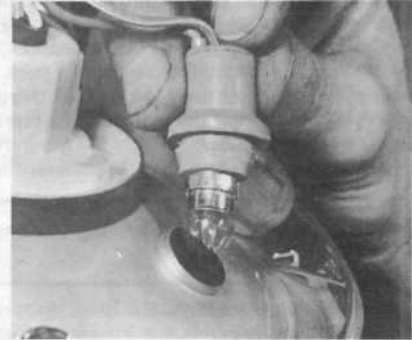
1.7f Pilot lamp bulbholder is a press fit in reflector ...
