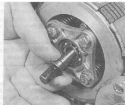
8.3b Clutch pushrod is now in one piece
