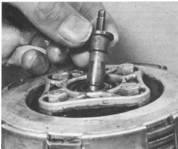
12.1a Remove the pushrod and pushrod seat
