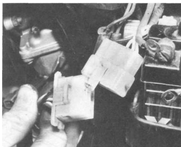
5.8b ... then separate the generator output lead connector
