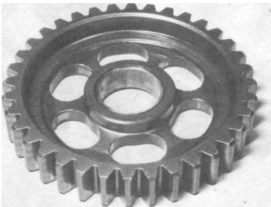
32.2j Bottom gear pinion (36T) has renewable bush
