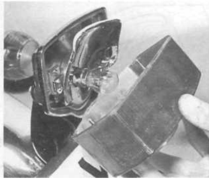
7.2 Tail lamp lens is retained by two screws
