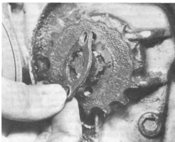
5.7 Release the locking plate to permit sprocket removal
