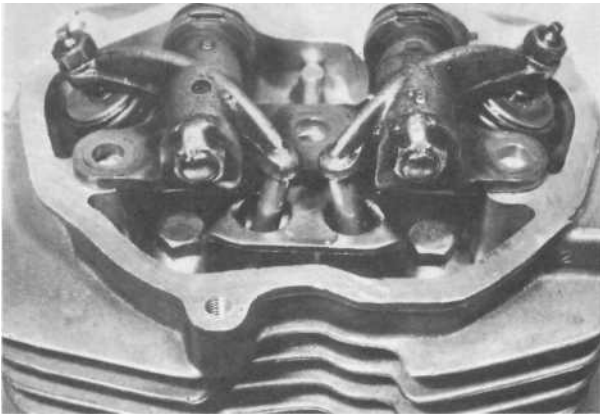
39.8a Refit pushrod guide and rocker assembly ...
