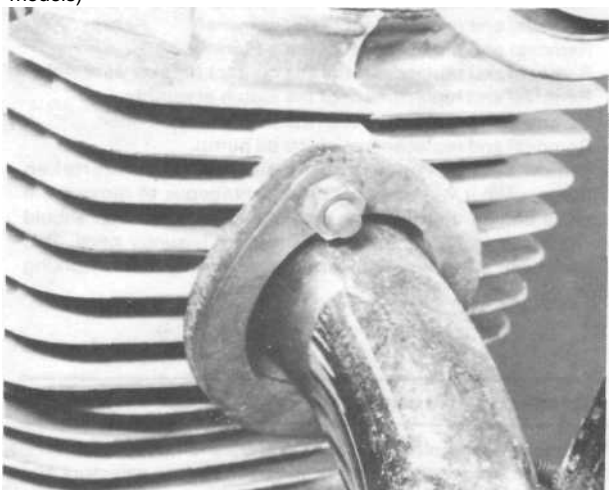
5.6a Remove exhaust pipe flange followed by .
