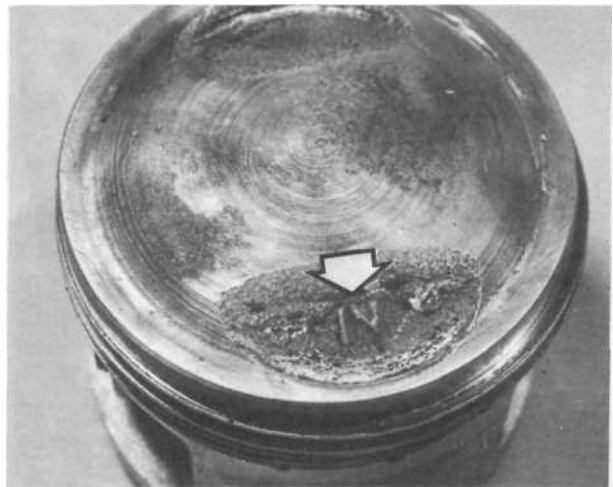
39.2 Cutout for inlet valve is marked appropriately
