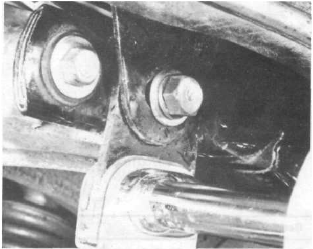
5.3 Seat is retained by two bolts at rear
