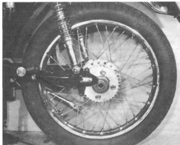
9.3c Wheel can be removed from frame
