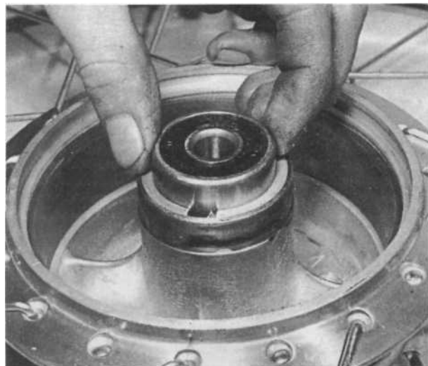
6.3b Bearing sealed surface must face outwards
