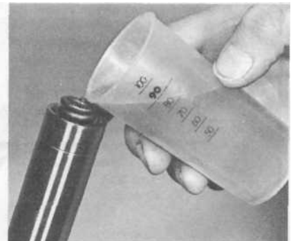
21.3b Refill fork leg with exactly the correct amount of oil
