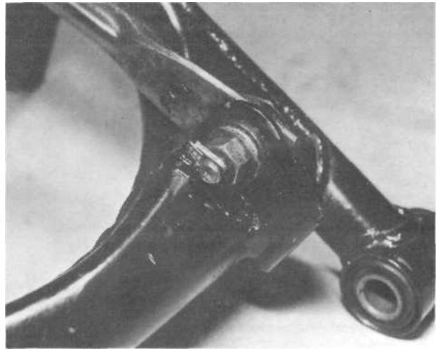
1 1.6 Check that torque arm mounting is secure
