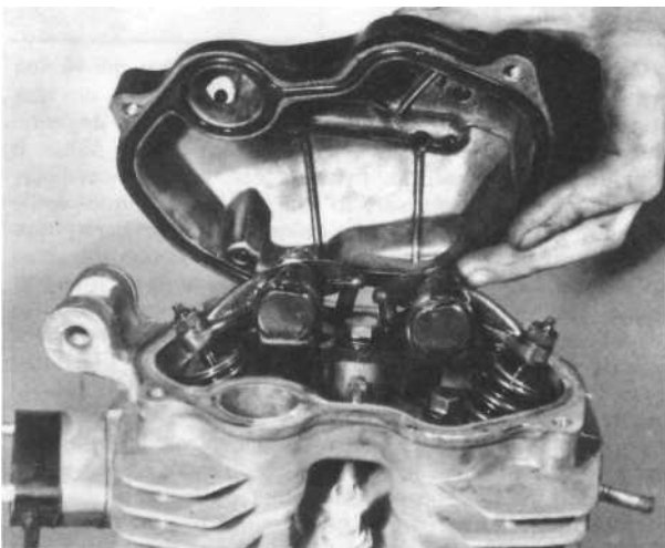
7.2a Remove the cylinder head cover to expose the valve gear
