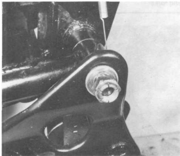
1 1.4a Slacken and remove pivot shaft nut
