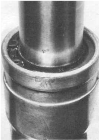
7.2a Remove seal retaining circlip
