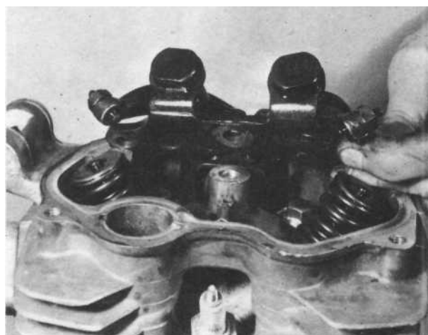
7.2b Release the three mounting bolts, and lift rocker assembly away as a unit
