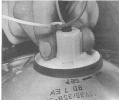
1.7d Headlamp bulb removal - procedure is similar to earlier models
