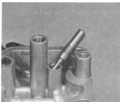
13.7a Carburettor jets are the same as earlier models - note removable pilot jet
