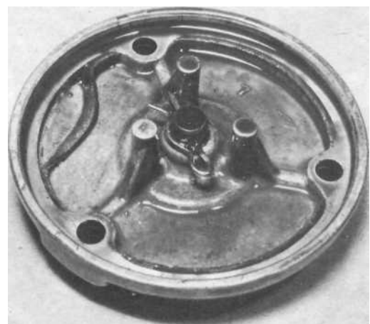
13.1 Centrifugal filter can be dismantled for cleaning
