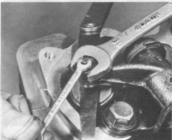
39.9 Adjust valve clearances, then refit cylinder head cover
