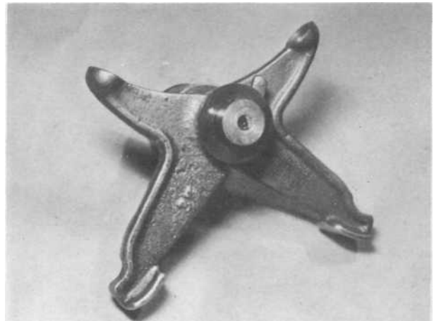
26.3 Check fit of followers on pivot shaft — note thrust washer
