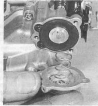
13.2a Pump cover is retained by three screws - note coil spring and valve in centre of cover
