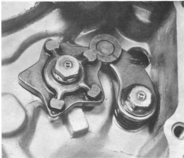
35.2c Fit camplate and tighten bolt
