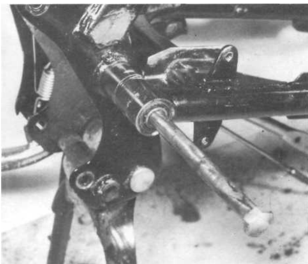
1 1.4b ... and withdraw the pivot shaft
