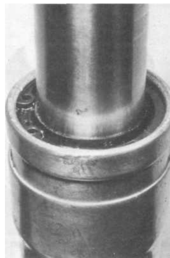
7.6e Renew seal and replace the circlip
