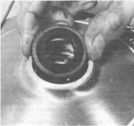
6.4 Renew seals together with bearings
